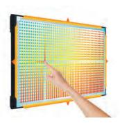
each touch event breaks two beams, giving an X and a Y coordinates. This corresponds to determine the location of the area on screen.
